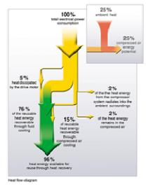
100 percent of the electrical energy fed to a compressor is converted into heat. With water cooled rotary screw compressors, up to 96 percent of that energy can be reused.
