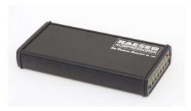
Compressed air audits using modern data-loggers (image) are easy to carry out and provide invaluable information regarding compressed air system efficiency and optimisation potential.
